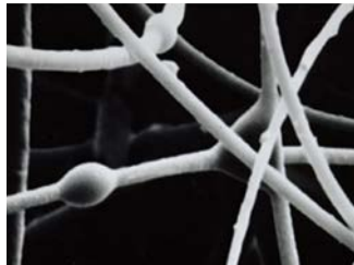
MERV 15 vs. MERV 8 media under 2000x magnification
