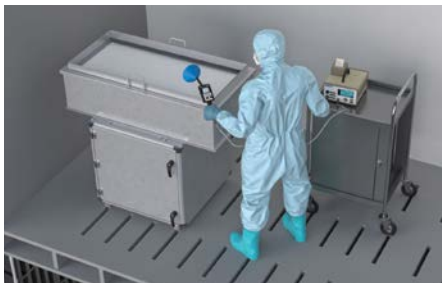
Bench testing of a HEPA/ULPA filter
